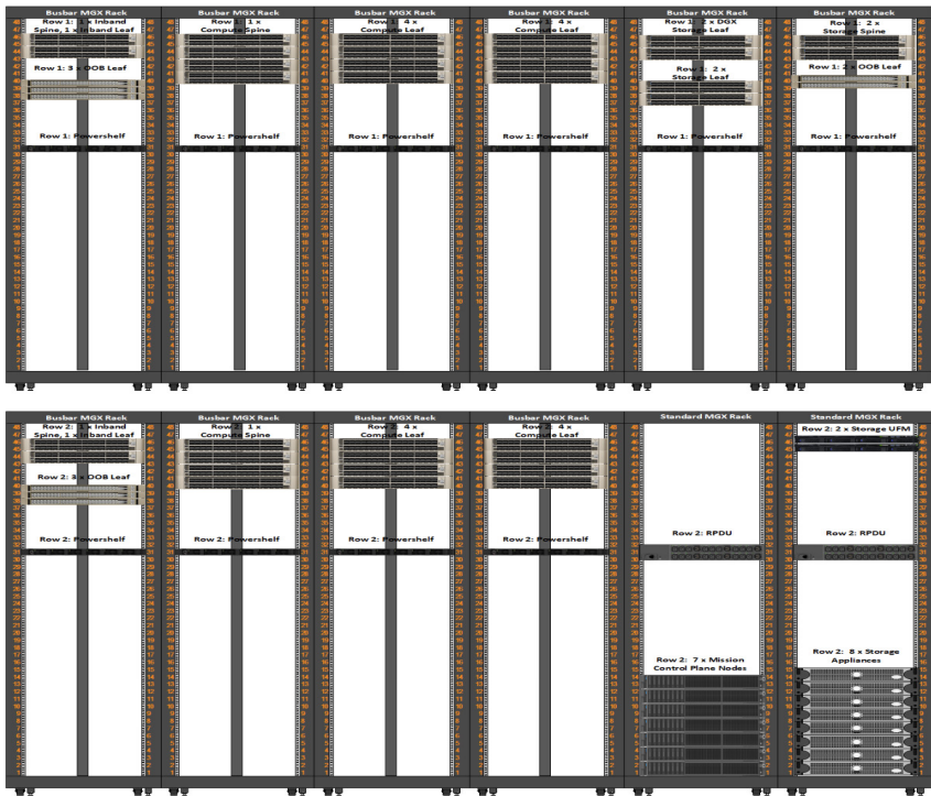
FIGURE 2 Example management rack configuration with networking switches, management servers, storage arrays, and UFM appliances (sizes and quantities will vary depending upon models used)
