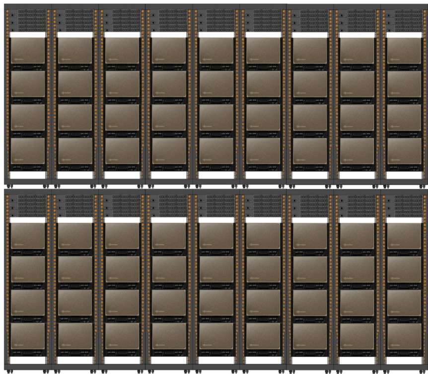
FIGURE 3 72 NVIDIA DGX B300 PS systems in standard racks each with three 2U rack power distribution units (PDUs) for maximum redundancy (you may need to reduce the number of DGXs hosted on the same rack depending on your data center’s capability)
