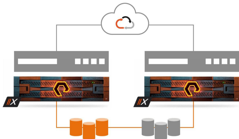
FIGURE 2 Technology overview of the ActiveCluster for SQL Server solution: Pure1 Cloud Mediator mediating between FlashArray systems to provide high availability for SQL Server data replicated between two sites
