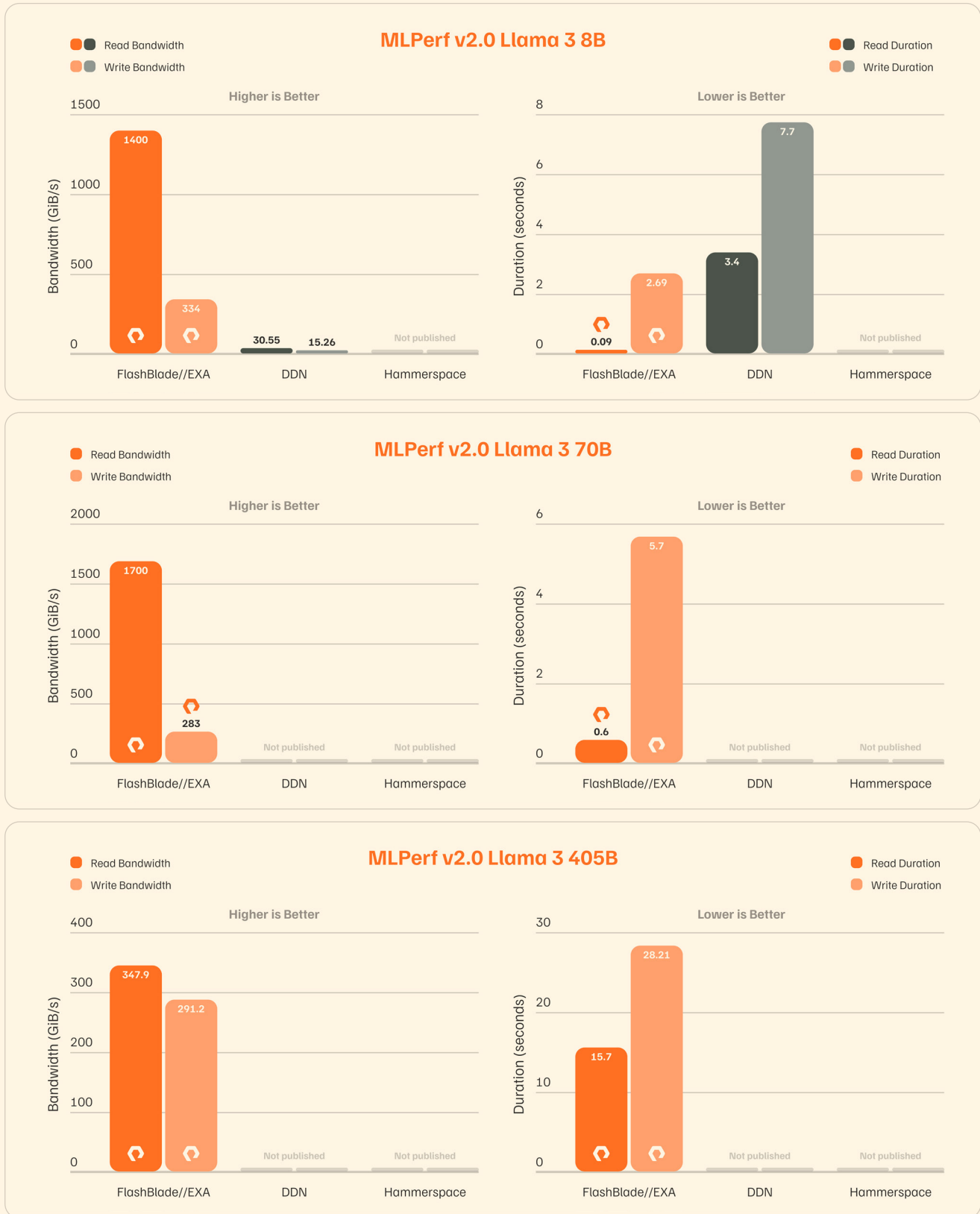
FIGURE 8 Summary of checkpoint benchmark tests comparing FlashBlade//EXA to best published Hammerspace and DDN results | Result not verified by MLCommons Association | Highest recorded reference
