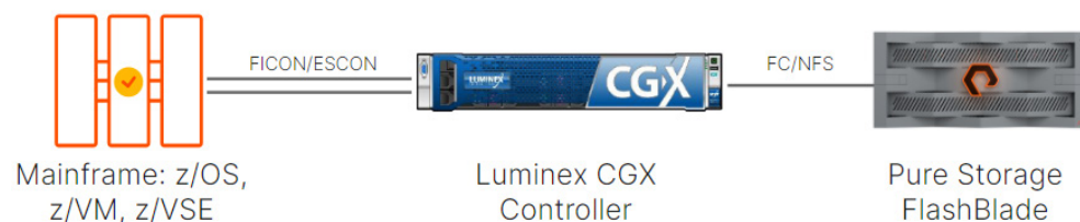
FIGURE 1 A basic virtual tape conceptual diagram. The mainframe is connected via FICON/ESCON to the Luminex GCX which emulates tape drives. The “virtual tape” data is stored on the Pure Storage device.
